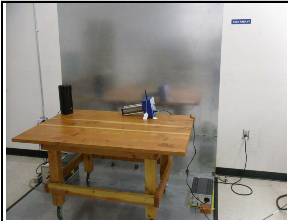
Test Setup Photo 1 – Conducted Emissions – Generator
